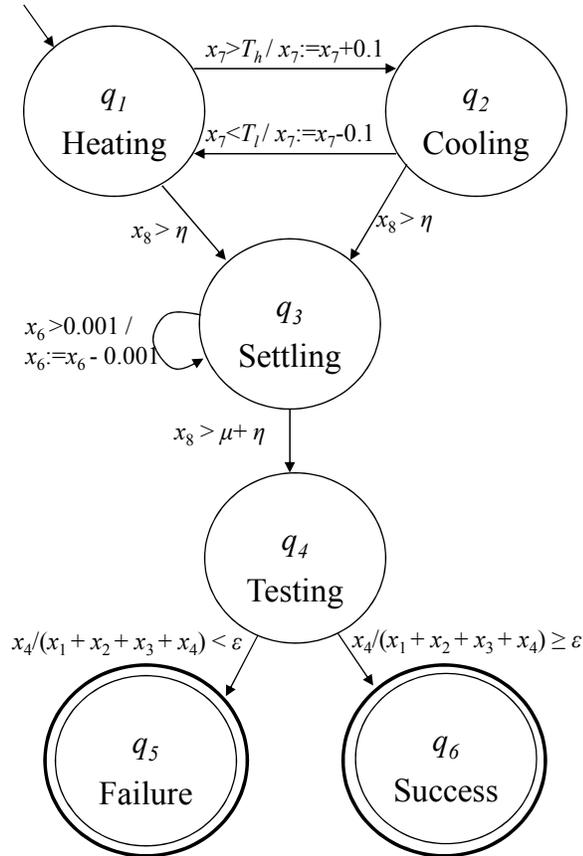
**Figure 6.** SHS model of biodiesel production system
