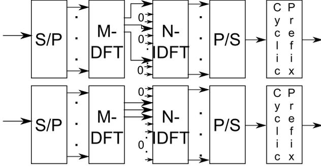
Fig. 2. Illustration of IFDMA (upper) and LFDMA (lower) signal flow
