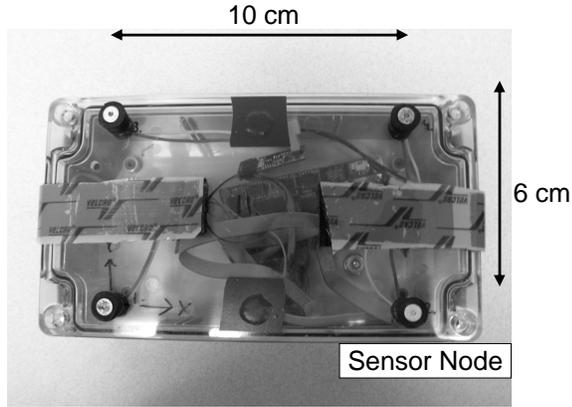
Fig. 9. Audio sensor node
