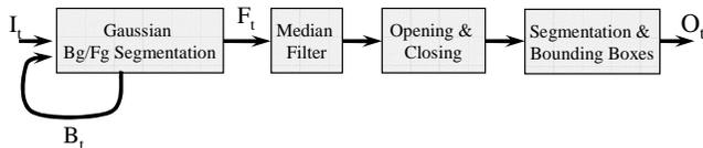
Fig. 10. Data-flow diagram of real-time moving object detection
