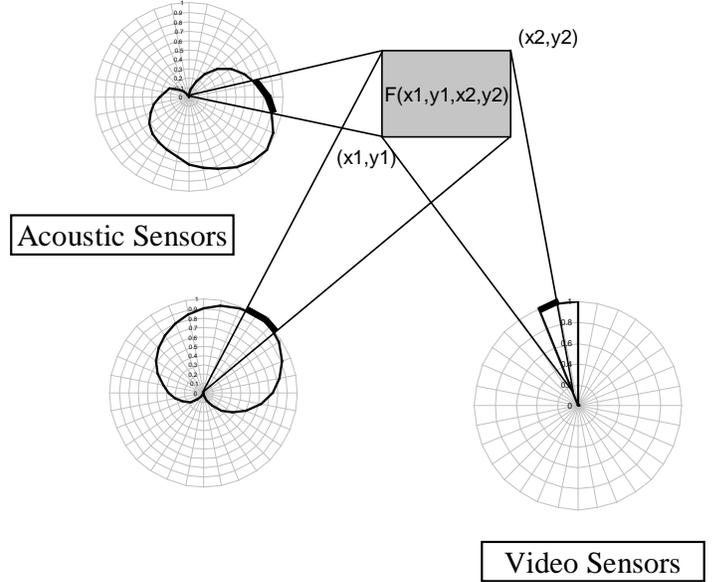
Fig. 11. Multi-modal sensor fusion. The sensing region is divided into rectangular regions and the consistency function is calculated for each region using acoustic and video data.
