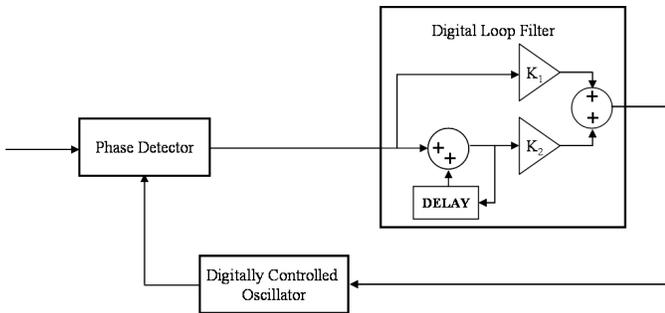
Fig. 2. Phase-locked loop
