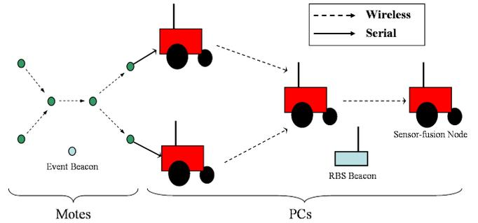
Fig. 3. Our sensor network testbed. Arrows indicate communication flow.
