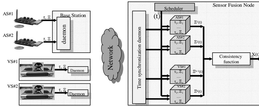
Fig. 12. Multi-modal tracking system architecture
