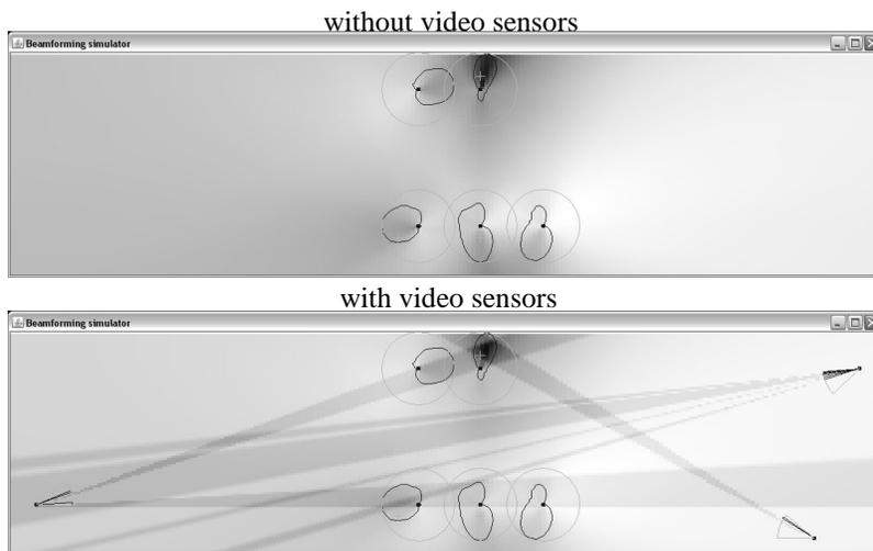
Fig. 15. Consistency function for multiple speakers
