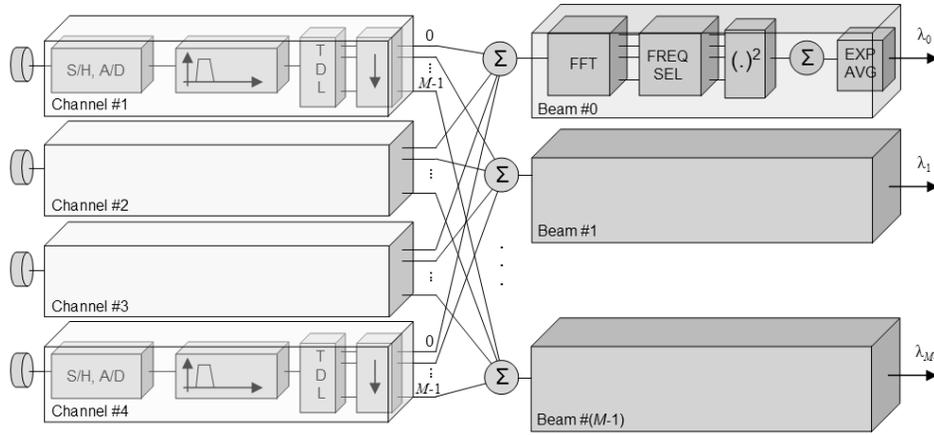
Fig. 7. Data-flow diagram of the audio beamforming algorithm
