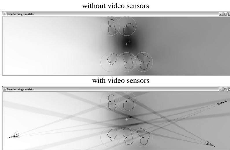
Fig. 13. Consistency function for a speaker inside the network
