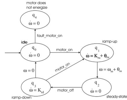
**Figure 3:** Hybrid model for the feed motor.
