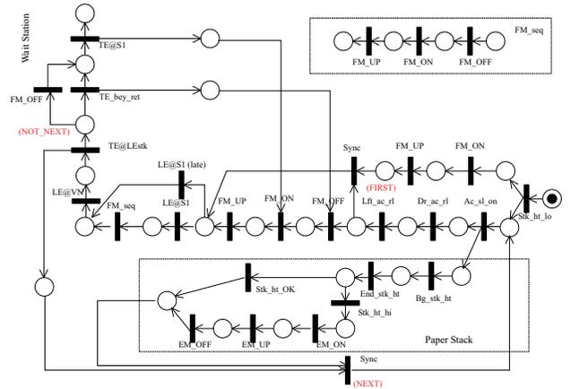
**Figure 7:** Petri net model of the paper feed system.
