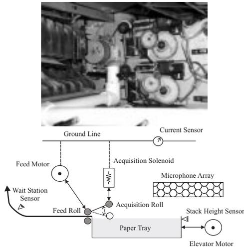
**Figure 2:** Paper feed system of the Xerox DC265 printer.
