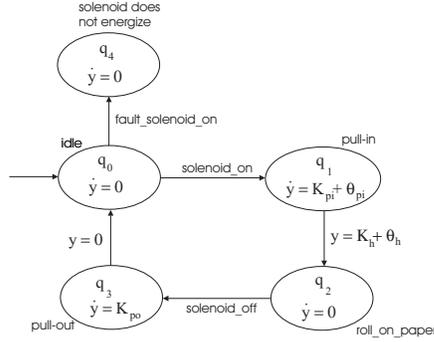
**Figure 4:** Hybrid model for the acquisition solenoid.
