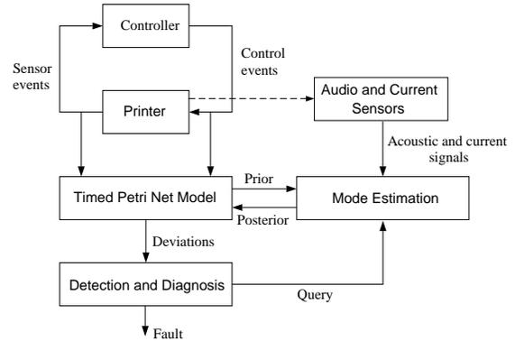
**Figure 1:** Architecture of the prototype diagnosis system.
