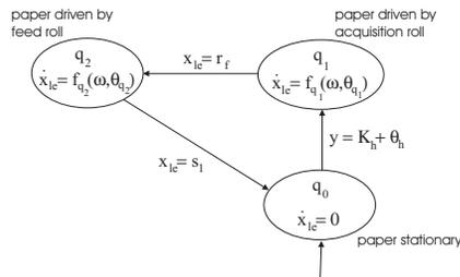
**Figure 5:** Hybrid model describing the paper motion.
