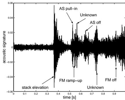
**Figure 8:** Acoustic signal for a one-page printing operation of DC265 printer.
