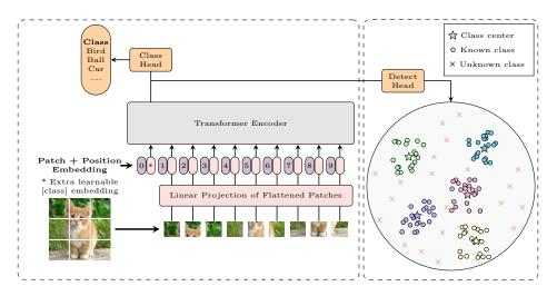
Fig. 2. Proposed architecture for open set recognition. Left: A ViT model to perform classification task for known classes; Right: A detection head attached to ViT to perform novelty detection for unknown classes
