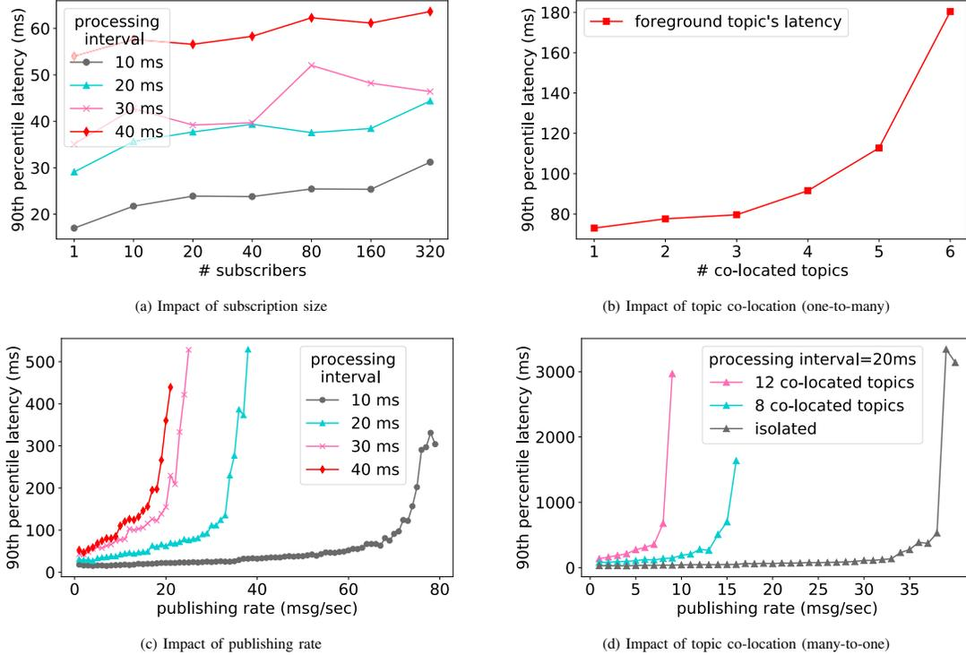
Fig. 1: Sensitivity analysis for latency modeling
