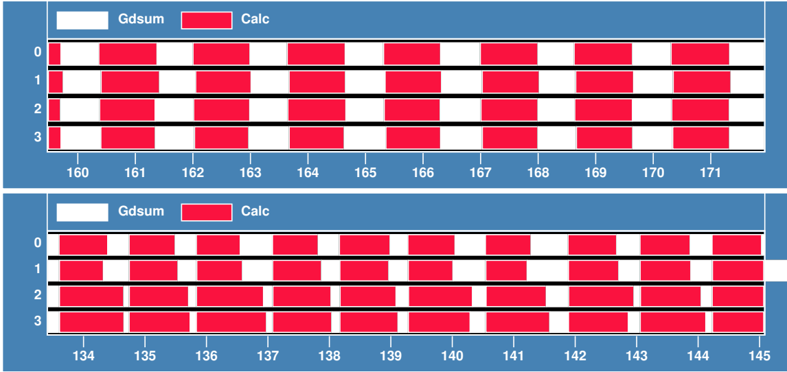
Figure 4: A comparison of computation (Calc) and global summation (GDSUM) during Davidson iterations: top IBM, bottom DEC.
