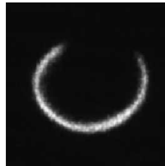
Figure 1. Axial integrated image of the concave H_2-N_2 /air opposed tubular flame at X_F=18.8\% , K=53 \text{ s}^{-1} , R_s \approx 6.5 \text{ mm} (upper part of the image is blocked by the inner nozzle).
