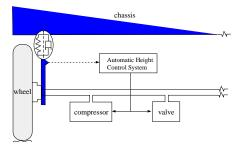
Fig. 1. Automatic height control system
