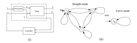
Fig. 5. (i) Hybrid system regulator, (ii) Controller
