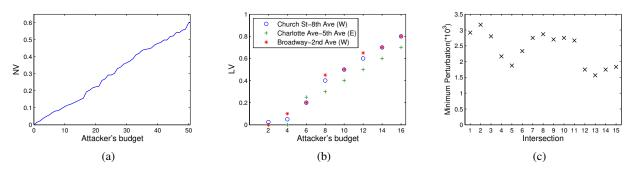
Fig. 5: (a) Network vulnerability as a function of attacker's budget in the case of worst-case network attack. (b) Lane vulnerability as a function of attacker's budget in the case of worst-case lane attacks. (c) Minimum perturbation needed to reduce the service time of each intersection by at least 50%, in the case of risk-averse target accumulation attack.
