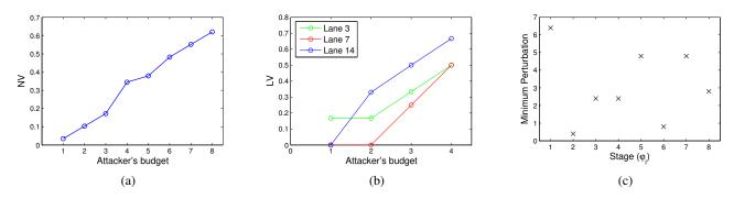
Fig. 3: (a) Network vulnerability as a function of attacker's budget in the case of worst case network attack. (b) Lane vulnerability as a function of attacker's budget in the case of worst case lane attacks. (c) Risk-averse target attack. The attacker's goal is to reduce the service time fractions to 0.05 by making the minimum perturbation.
