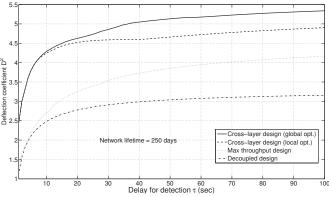
Figure 11. Deflection coefficient as it varies with the delay for detection.
