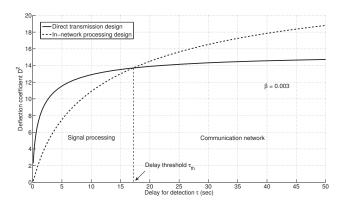
Figure 13. Deflection coefficient for direct transmission and in-network processing designs.
