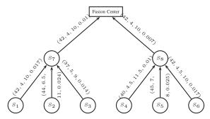
Figure 8. Tree detection network for the example problem. Labels on each edge represent  $\mu_c, \sigma_c, e$  (in mJ), and Signal to noise ratio, respectively, for each source sensor.
