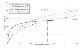
Figure 14. Variation of detection threshold with quantizer parameter  $\beta$ .
