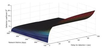
Figure 9. Deflection coefficient as it varies with the network lifetime and delay for detection.
