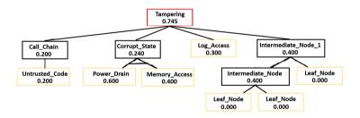
Fig. 2. Component attack tree for Tampering risk of a sensor
