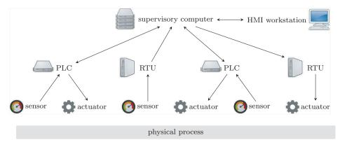
**Figure 1.** Example cyber-physical system. Arrows represent flows of sensor data and control signals.
