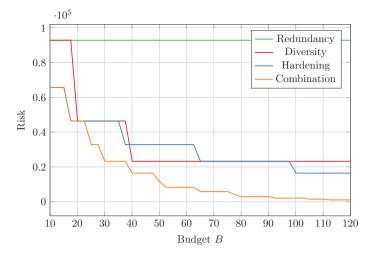
**Figure 3.** Security risk in the water-distribution network when investing only in redundancy, only in diversity, only in hardening, or in their combination.
