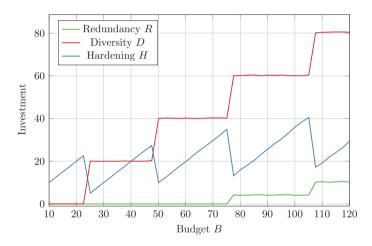
**Figure 4.** Optimal combination of redundancy, diversity, and hardening investments in the water-distribution network.
